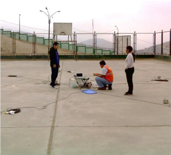
Fig. 6. Microtremor array test in the Ventanilla district.
